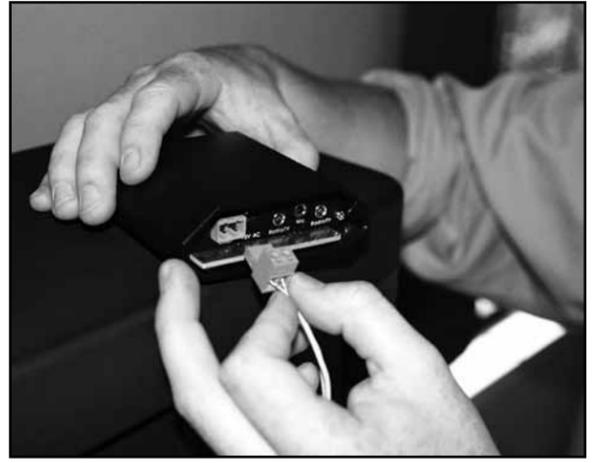
15 Plug one end of the cable into the **Radio/TV** connection on the amplifier
