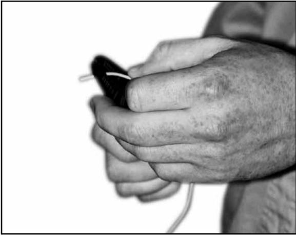
13 Remove the connector from the amplifier, insert cable ends, and tighten screws
