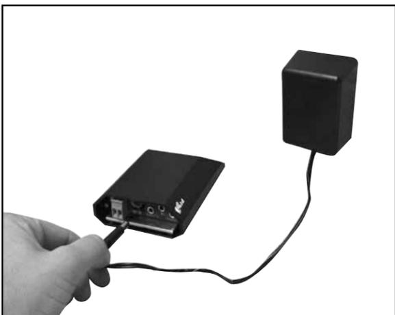
Typical an indication light on the front of the loop eluminates should go on. Adjust the output strength on the front of your loop to the desired level.
