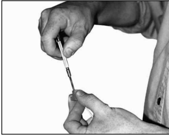
14 Replace the connector of the cable loop into the back of the amplifier unit
