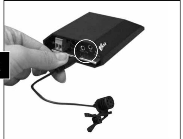
If the sound source cannot be attached to the teleloop using the Line Out connection, place the microphone in front of the television or stereo speaker.
